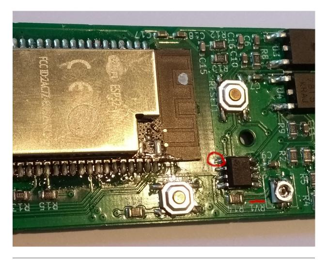
**Note:** Although most boards do not have it yet, image quality for partial updates can be improved by adding a (at least) 4.7uF capacitor between VCOM and GND. When adding this capacitor, take care with the polarity as VCOM is negative!
